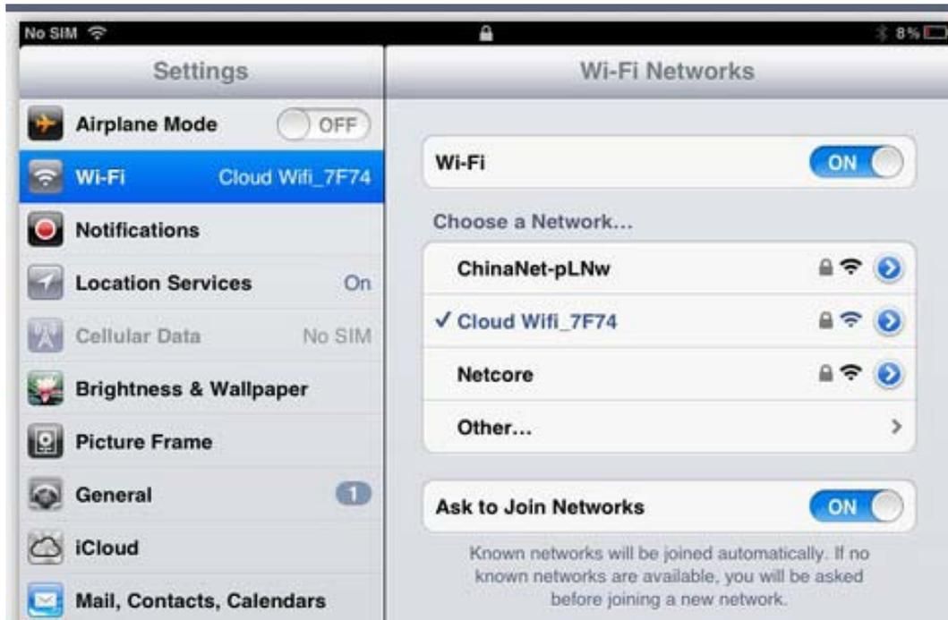
Step 3: View and set network parameters. Click the “>” button on the right of connected wireless router. Then, the parameter setting page of wireless network pops up (the router starts the DHCP server by defaults and recommends the use of DHCP).
