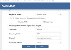
Step 6.1.4: After configuration, please connect the new WiFi signal of the repeater and check if you could get Internet. The management page password should be same as the Wi-Fi password of the repeater. Step 6.1.5: Put your repeater in an ideal location where there aren't
