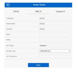
Enter the Device wireless parameter. It's recommended that you rename an SSID, choose a Security Mode and enter a Wi-Fi Password.
