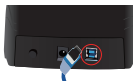
Connect the other side of the USB cable in the HDD case
