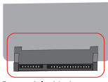
Be careful with the connector pins, watch the position when connecting the HDD
