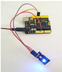
Done uploading the code, you should see the RGB LED flashing with different colors.
