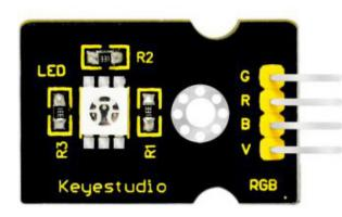
This is a full-color LED module, which contains 3 basic colours, red, green and blue. They can be seen as separate LED lights. After programming, you can turn them on and off by sequence or can also use PWM analog output to mix three colors to generate different colors.
