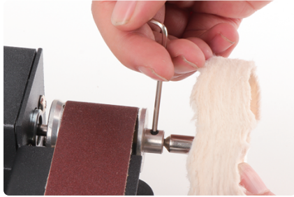
5. Insert the cloth wheel and tighten the small screw.
