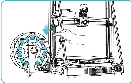
③ Remove the old filaments by pulling them out from the back of the machine to replace with new ones.
