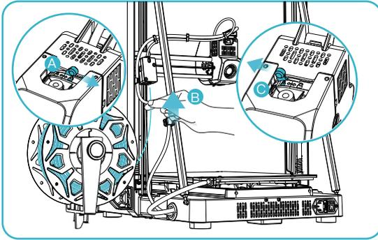
① A. Unlock the DIP switch; B. Insert the filament into the deepest part of the Teflon tube until it cannot be moved; C. Lock the DIP switch.
