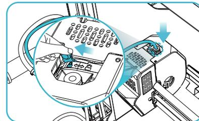
⑥ Lock the DIP switch, and insert the Teflon tube into the upper joint of the extruder kit.
