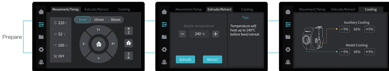
\* You can configure functions such as axis movement/temperature control, extrude/retract, and fan cooling through the preparation interface.
