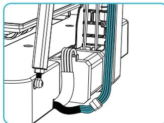
5 Connect the limit switch cable;
