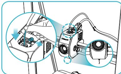
⑤ Unlock the DIP switch and thread the filament into the extruder kit until the filament is extruded from the nozzle;
