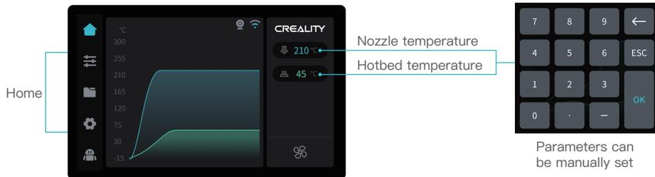
\* You can configure functions such as extruder temperature and hotbed temperature through the homepage;
