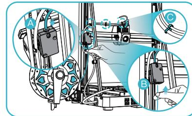
④ A. Connect the Teflon tube to filament runout sensor; B. And thread the filament into filament detection port until it passes through the Teflon tube; C. Fix the Teflon tube with extruder cable with cable clips,
