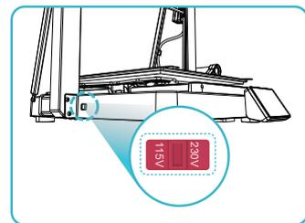
6 Select the correct voltage mode based on the local power grid voltage.
