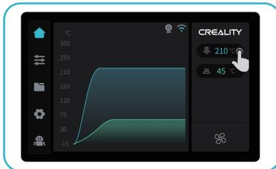
① Input the nozzle temperature on the screen and wait for it to heat up to the target temperature;
