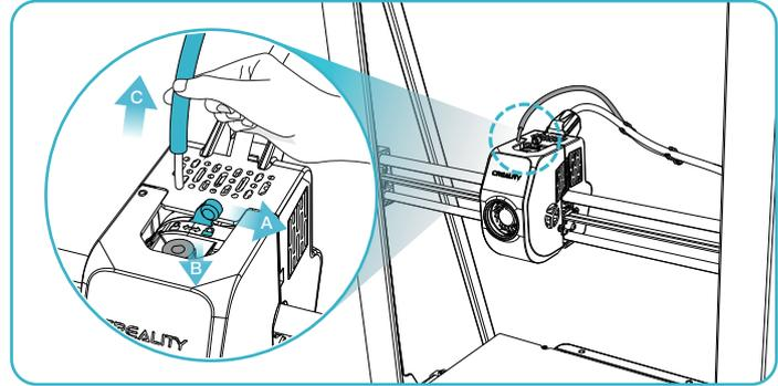
② a. Unlock the dip switch; b. Hold the Teflon tube connector above the extruder; c. Pull out the Teflon tube;
