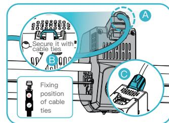
2 A. Connect the extruder kit first; B. Fix the extruder cable with cable ties; C. Install the extruder cable cover;
