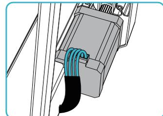
4 Connect the X&Z-axis motor (right);
