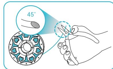
② Cut the front of the filament at 45° and break it off straight;
