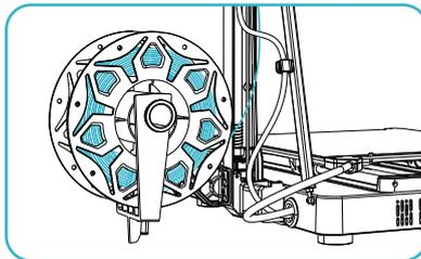
③ Arrange the filaments as shown in the picture, and then install the anti-tangle material rack;
