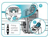
2 A.Connect the extruder kit first; B. Fix the extruder cable with cable ties; C. Install the extruder cable cover:
