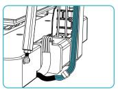
5 Connect the limit switch cable;
