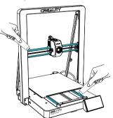
Optical axis area of X & Y direction
