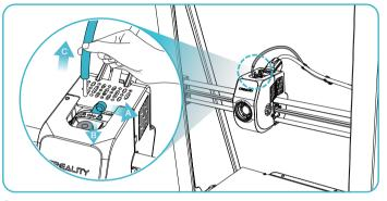
${\textcircled{2}}$  a. Unlock the dip switch; b. Hold the Teflon tube connector above the extruder; c. Pull out the Teflon tube;
