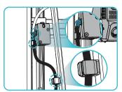
1 First, clip the wire into the wire clip, and then connect the filament runout sensor line:
