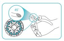
$\ensuremath{\text{@}}$  Cut the front of the filament at  $45^\circ$  and break it off straight;
