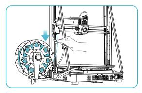
$\ensuremath{\ensuremath{\Im}}$  Remove the old filaments by pulling them out from the back of the machine to replace with new ones.
