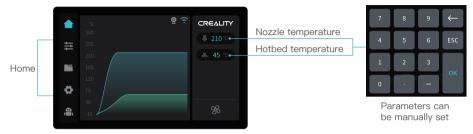
\* You can configure functions such as extruder temperature and hotbed temperature through the homepage;
