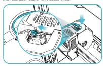
$\ensuremath{\widehat{\otimes}}$  Lock the DIP switch, and insert the Teflon tube into the upper joint of the extruder kit.
