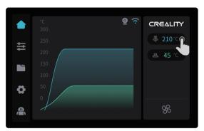
① Input the nozzle temperature on the screen and wait for it to heat up to the target temperature;
