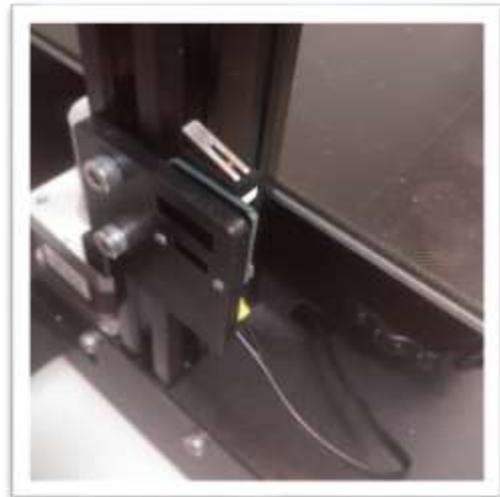
(right: incorrect positioning of the z-axis sensor)
