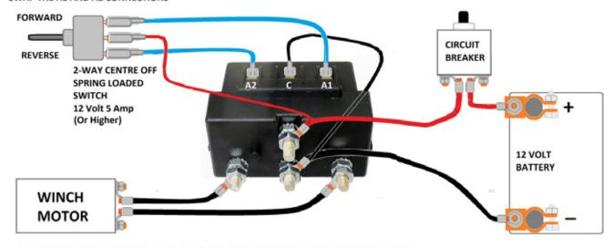
**CONNECTIONS FOR 2-WIRE WINCH MOTORS**
