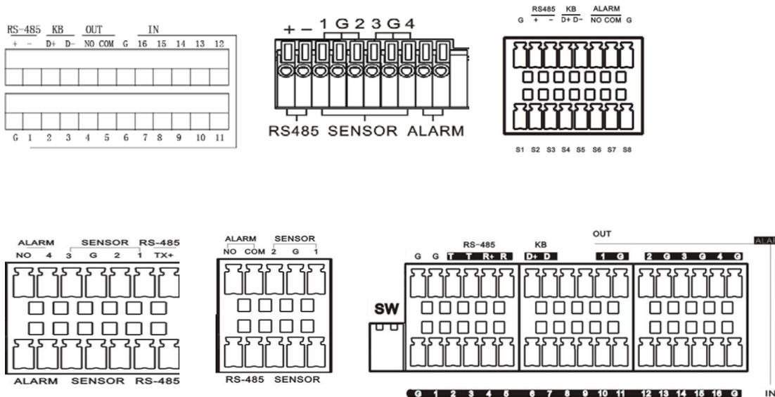
**Alarm input:** Check your purchased alarm device and connect a G (GND) foot to the port marked with “-” and connect the alarm channel to the port marked with “+”.
