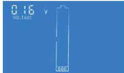
Figure 5: cut-off voltage setting interface(low bit) Figure 6: cut-off voltage setting interface(high bit)
