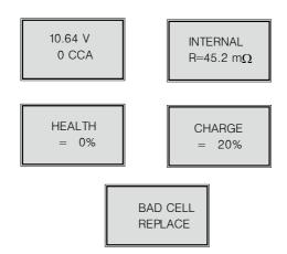
Battery interior damaged, broken cell or short circuit, replace battery. (Healthy=0, Voltage<12.4V, Electric Current=0A or OCCA)
