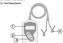
1.LCD DISPLAY-Indicates test results. It is a backlit 2-line display with 8 characters on each line
