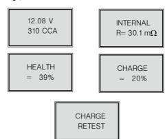
Unstable battery shall be recharged and retested to avoid error. If same test result appears after recharge and retest, the battery is regarded as damaged, replace the battery.
