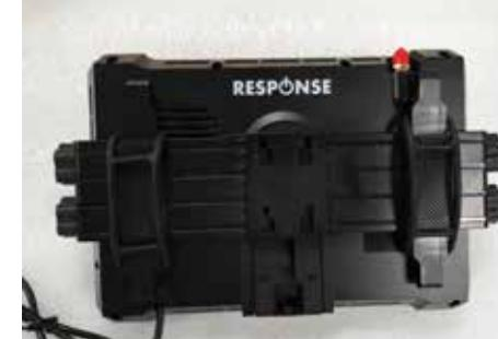
**Install foldable & extendable bracket(No.10) on 7 inch monitor**
