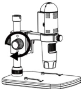
**Rotate Wheel 7 to lock or release the movement!**
