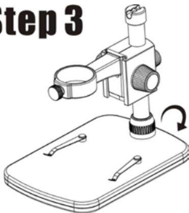
Rotate Wheel 10 to fix the pole on the stage!
