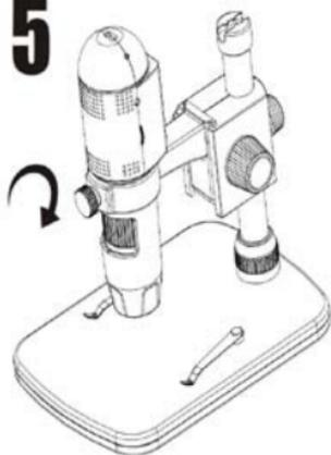
Rotate Wheel 11 clockwise to fix the microscope on the ring.
