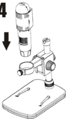
Put the microscope into the ring of the stand!
