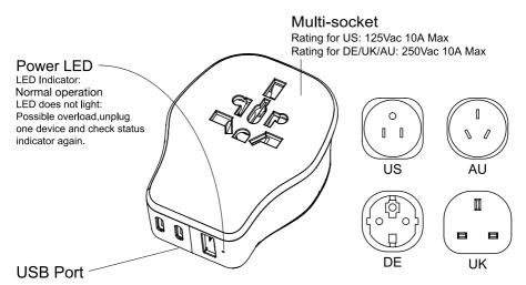
USB-C output: 5.0V==3.0A | 9.0V==2.22A | 12.0V==1.67A 20.0W USB-A output: 5.0V==3.0A | 9.0V==2.0A | 12.0V==1.5A 18.0W USB-C1+C2+A1 output: 5.0V==3.0A 15.0W Max
