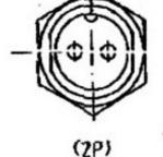
RATED VOLTAGE: 32VDC RATED CURRENT: 7A CONTACT RESISTANCE : 0.005 OHM AND LESS FOR EACH CONTACT WATER RESISTANCE : 1P55
