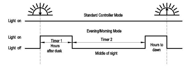
The MP-3739 recognizes days and night based on the solar array voltage. NLF will start when the PV(Voltage) < 10V for a period of time.
