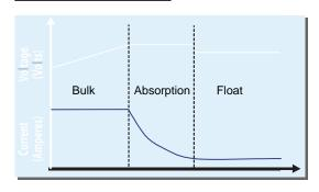
**Bulk:** This is the first stage where the battery is in a low charge state, where it receives the majority of its charge. During this stage the battery brought to about 85-95% capacity getting 100% of the available solar power.
