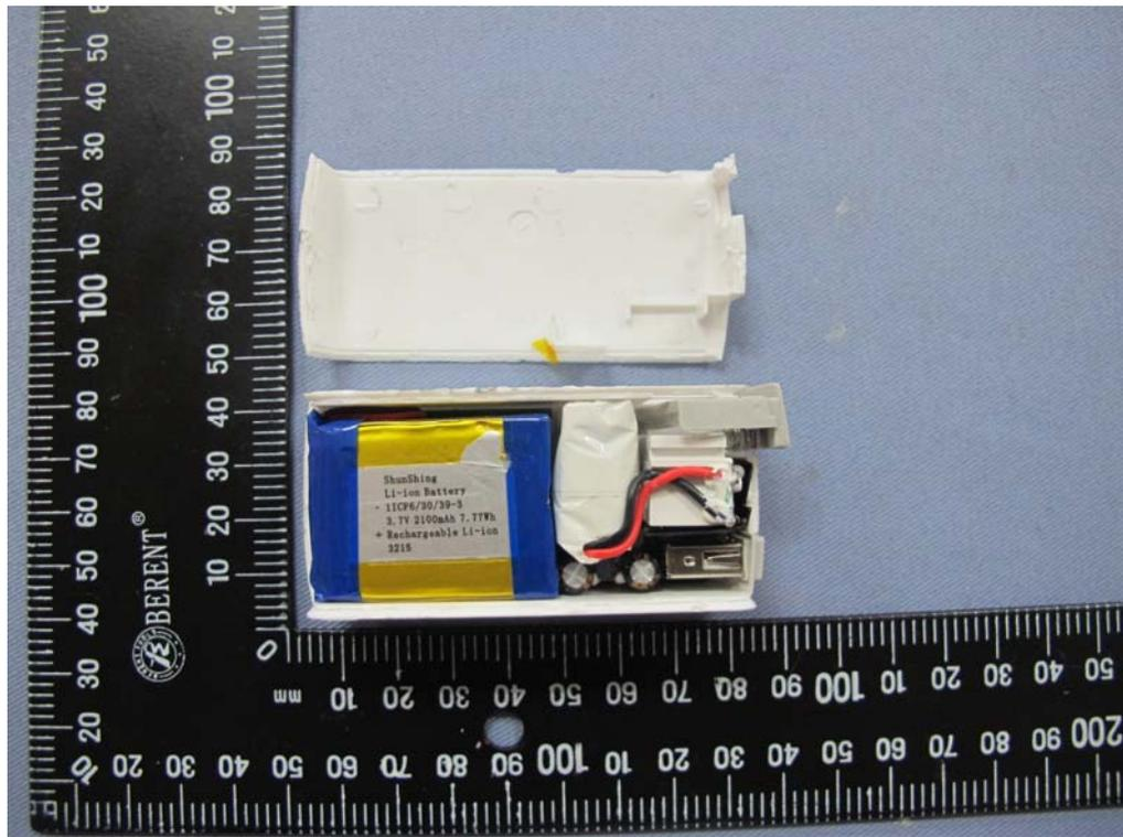
Figure 3 Internal view of power bank
