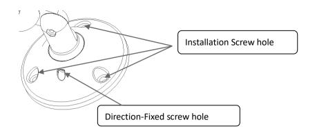
2. You can rotate the bracket to adjust lens direction. See below photo
