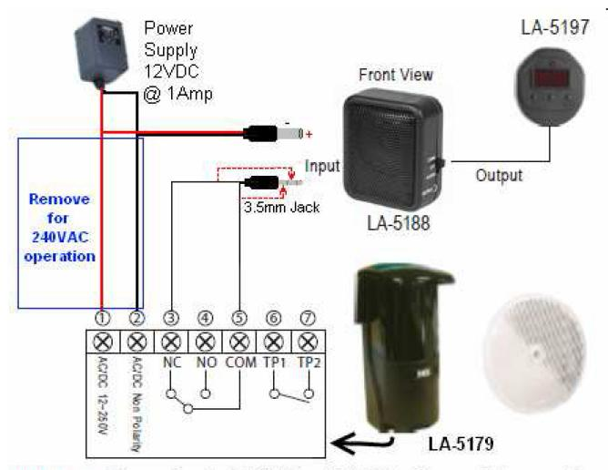
WARNING: If powering the LA5179 from 240VAC (mains supply) remove the two wires from terminals 1 and 2 and connect to mains supply.
