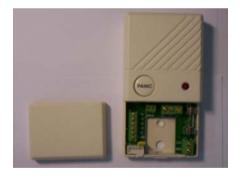
☑Step 3: Wiring all needed cables through wiring hole in relay box: open relay box (use coin), see the wiring hole and several terminal blocks surrounded on the green circuit board with printed indicators:
