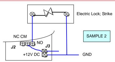
Relay Box (open case) \*All cables wire through the hole on back case.
