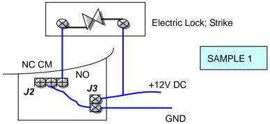
Relay Box (open case) \*All cables wire through the hole on back case.
