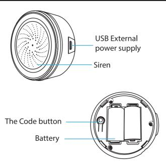
Notice: Pleases use USB power supply, the backup battery can only work for two days. Plug in the USB power supply and load the battery at the same time, then the sensor will work in priority.
