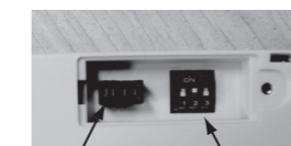
House Code Jumpers Chime Dip Switches Sensor Jumpers and Dip Switches
