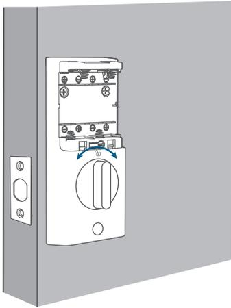
Make sure the deadbolt is retracted and the thumb turn knob is on the 'unlock' position, check if the deadbolt moves properly by turning the thumbturn.
