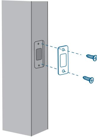
Make sure the depth of the latch hole on door frame is deep enough (25.4mm/1"), otherwise the calibration might be failed during the setup.
