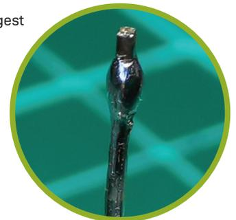
You should also tin the point where the cathode will join the next layer, which is the 90° bend where the lead goes from horizontal to vertical.
