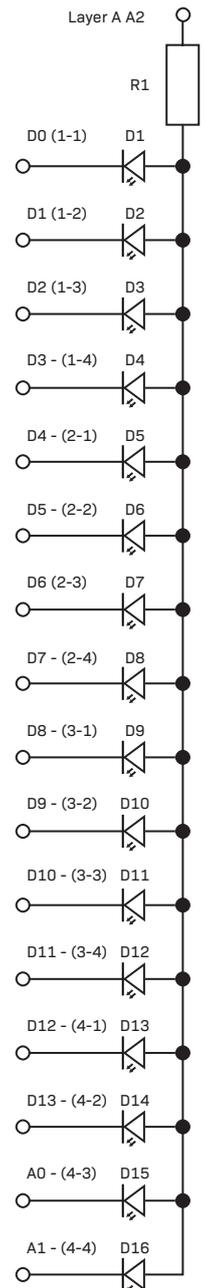
This is less than the absolute maximum of that LED, meaning it won't be destroyed and will be reasonably close to its absolute brightness. With that said, in practice, the difference in apparent brightness between a few LEDs per layer and all 16 LEDs per layer illuminated, is not all that apparent when the project is running.
