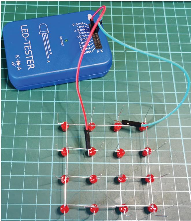
This layer was a conceptual layer and not the same design as our final design. We are simply using it here to demonstrate how you can use the LED tester to test the layer functions correctly.
