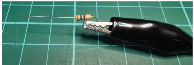
*Note: if your power supply does not have the ability to limit the current you can use a resistor on the cathode alligator clip like shown here. You simply touch the exposed end of the resistor to the cathodes of each LED. Note be very careful with this though. If*
