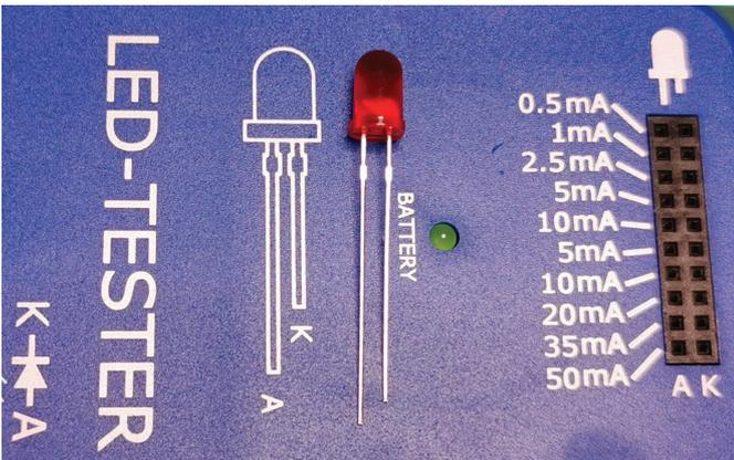
Once you have confirmed that the LED is working correctly, you can then carefully bend the LED's cathode leg, which is the shorter leg (also the side with the flat edge on the LED's rim). You will also notice a printed diagram of the LED and its anode (A) and cathode (K) on the LED tester.
