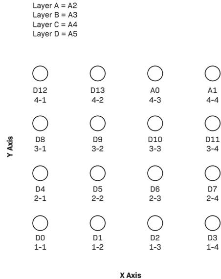
This shows the position of each LED, along with their corresponding pins. You can use the values silkscreened on the PCB to help orient the cube. i.e. (1-1) is the bottom left corner, while (4-4) is the top right, etc.
