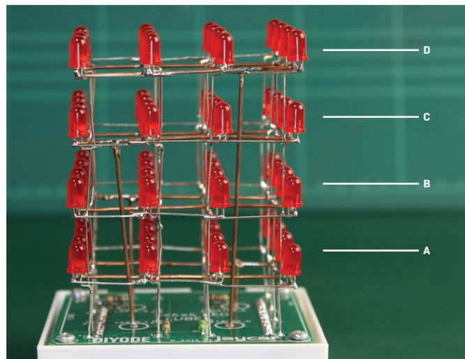
With the LED cube constructed, you can insert it into your Arduino Uno or compatible board (Hopefully you have the header pins already soldered onto the PCB).
