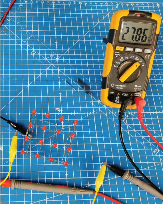
We left this test running on 5V for the duration of this project, and we saw no obvious reduction in output brightness (At the time of writing, it has been over 14 days or roughly 330 hours).
