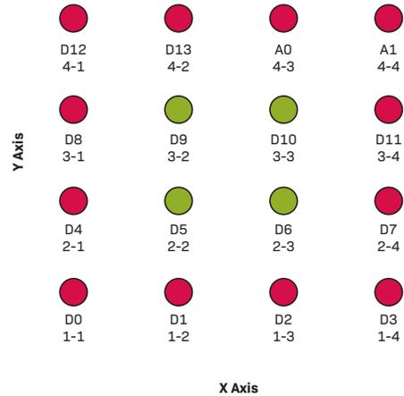
To illuminate the outer 12 LEDs, you need to pull the corresponding pins (shown in red) low for the following coordinates, using the key:
