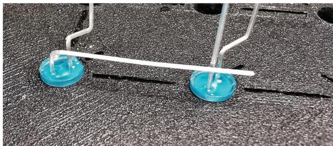
Once the first three LEDs are in place, start soldering the anodes together. This will help avoid the LEDs being accidentally misaligned if you bump them, etc.
