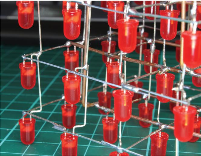
To join two layers, you first need to align the layer making sure the strengthening copper rods are all running in the same direction.
