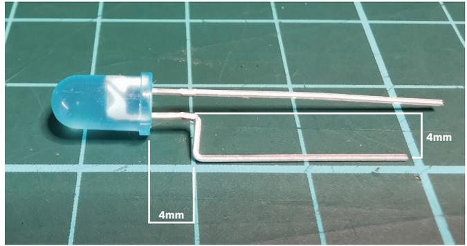
You need to bend this cathode leg so that it has two 90° bends, each about 4mm apart. To make these bends, we used a pair of long nose pliers to hold the leg where we wanted the bend, and then gently bent the leg at that point.
