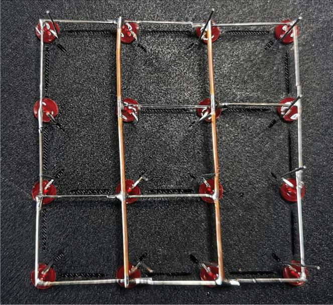
Pay attention to make sure that you are not shorting an LED's vertical anode to this wire. The wire may come close in some spots. Make sure you avoid any short circuits because these will cause a layer to not function correctly.
