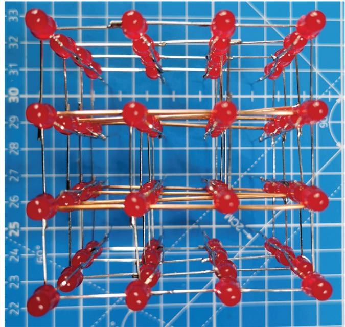
When you're done soldering the layers you should have a cube that resembles something like this. Note the middle two rows (horizontal) are closer together than the outer layers. These rows need to line up with the corresponding two layers on the PCB, as shown here.
