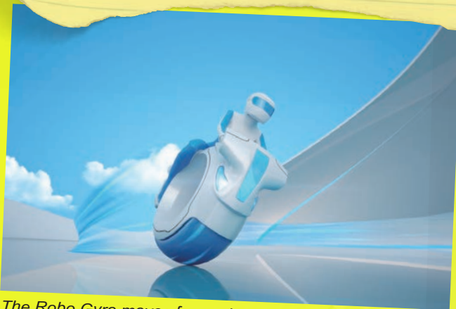
The Robo Gyro moves forward and keeps balance by using the engine and flywheel
