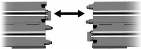
Insert the tracks together on a flat surface.
