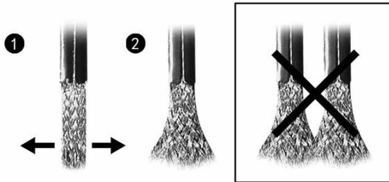
The brush located on the bottom of each car needs to be straight (fig 1.). If the brush has tangled, then stretch it out slightly so that it's completely straight.
