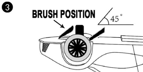
The brushes below each car need to be situated at an angle of 45° to run correctly.
