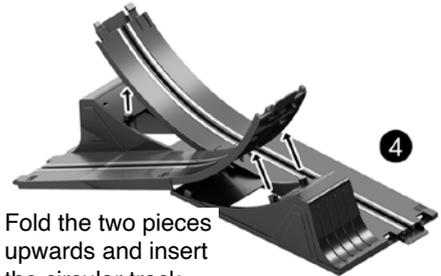
4 Fold the two pieces upwards and insert the circular track into the groove.
