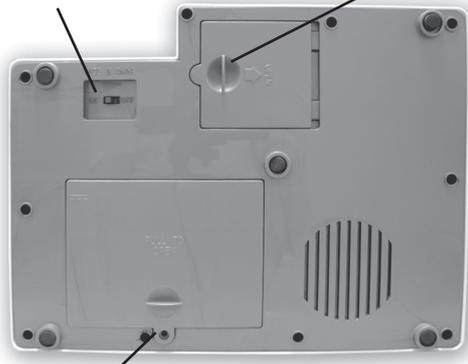
\*Remove screw at the bottom of machine to open battery compartment. (requires 3 "D" batteries)
