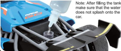
Note: After filling the tank, make sure that the water does not splash onto the car.
