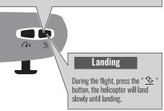
Don't operate the left stick during landing, otherwise the current command will automatically fail.
