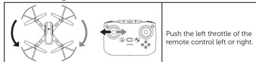
Push the left throttle of the remote control left or right.
