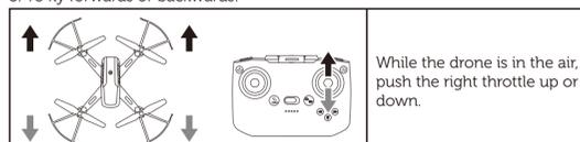
While the drone is in the air, push the right throttle up or down.
