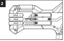
Insert 3 AAA batteries (not included). Make sure the batteries are inserted with the correct polarity.
