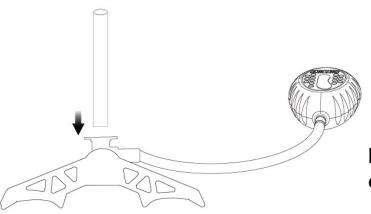
Insert the long tube to the top of the connector
