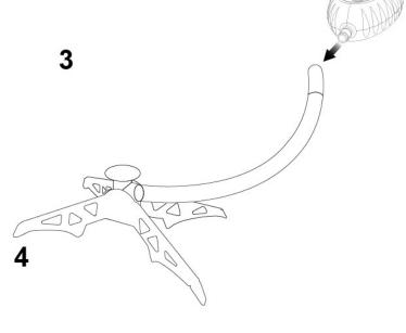
Insert the pump to the tube of the connector
