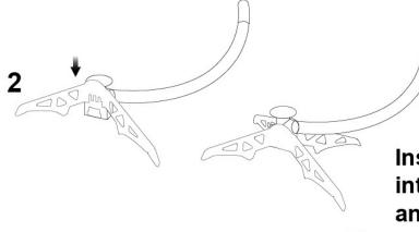
Insert the two bases into the square sockets in front and behind the connector
