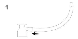
Connect the air tube into the right side of the connector
