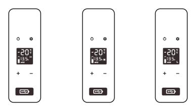
H should be set when the product is connected to car power, and M or L should be set when it is connected to a portable battery or other back-up battery. Because of the different output voltages between vehicles, the battery protection level can be set from H to M or from M to L if there is a voltage protection code F1 shown on the panel. The battery protection level should be set to H if the product will keep working after turning off the car engine, or the product may drain the battery.
