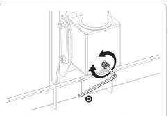
**Note:** If the display does not stop at your desired position, adjust the screws using the tools as shown.
