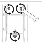
**Note:** Loosen the screws as shown and adjust the display to the desired angle, then tighten the screws.
