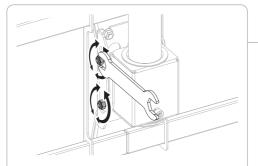
**Note:** Loosen the screws as shown and adjust the display to the desired angle, then tighten the screws.
