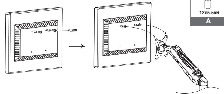
Recessed surface installation: Put spacers between headplate and monitor. Install the upper two screws and don't screw them tight. Leave some space and hang the monitor on the head plate.
