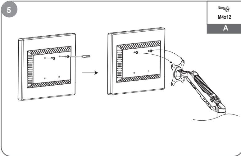
Flush surface installation: Install the upper two screws and don't screw them tight. Leave some space and hang the monitor on the head plate.
