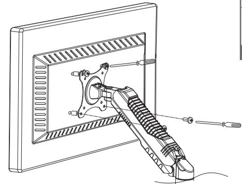
Recessed surface installation: Put spacers between headplate and monitor. Install the lower two screws and fasten the upper two screws.
