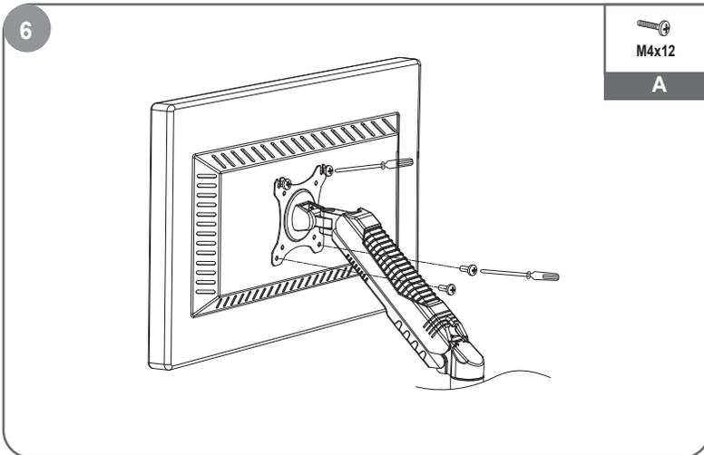
Flush surface installation: Install the lower two screws and fasten the upper two screws.
