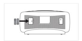
Replace the battery if the device is not used for a prolonged period of time (more than 1 month); Please take the battery out in order to prevent leakage of battery acid.
