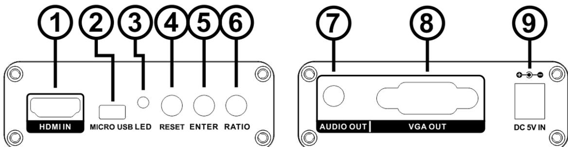
1. HDMI IN: This slot is where you connect the HDMI source output from DVD, PC or Laptop.
