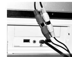
(1.3) After the transmitter and the audio cables are connected well, switch on the transmitter, the power indicator will be on. Choose a suitable place for the transmitter near the sound source (e.g. TV). Face the IR window of the transmitter to the receiving area. Adjust the audio source in working status and turn up its volume properly (when the transmitter is connected to a STB, DVD, PC, etc).
