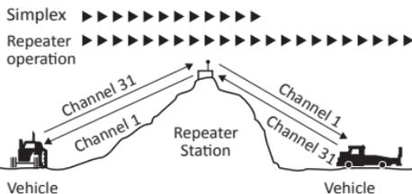
Duplex operation operates only on channels 1 – 8 or 41 – 48. When duplex is selected on these channels, the radio receives on that channel but actually transmits 30 channels higher. (See chart below).
