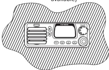
It is advisable to spend a little time selecting the best location for your TX4610. The mounting bracket can be rotated above, below or behind the radio enabling the radio to be mounted in a wide range of locations. In addition, an optional flush mounting kit allows the radio to be flush mounted in a panel or dashboard.
