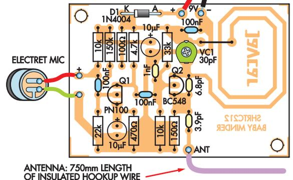
SHRTC212 and although its tracks provide the oscillator's resonating coil as well as making the circuit connections, it still measures only 59 x 41mm.
