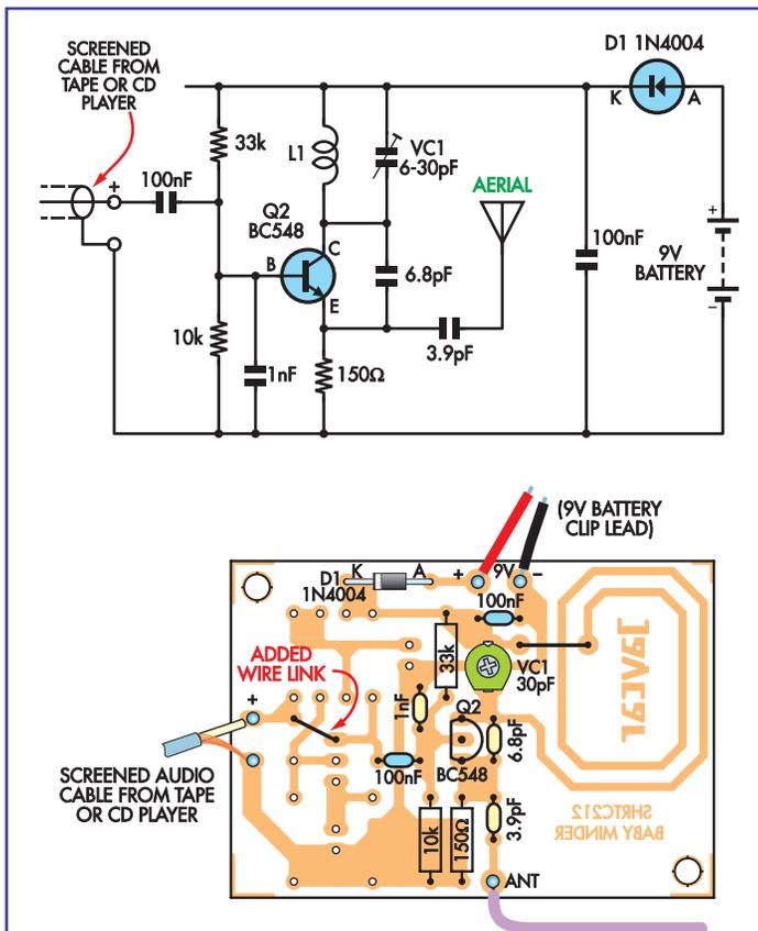
**Here's how to modify the FM Radio Mic so it can be used to feed audio from your tape or CD player into a hifi system via its FM tuner.**
