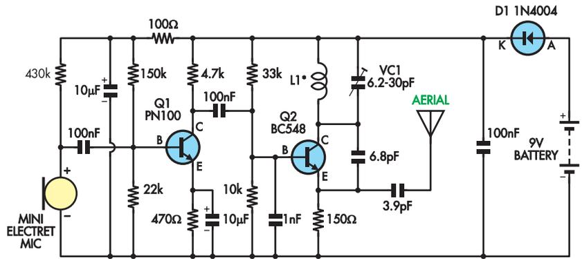
\*L1 FORMED FROM COIL OF TRACK ON PC BOARD
