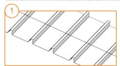
Determine where the roof mounts will be positioned and use a tape measure or chalk line to mark the roof.
