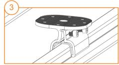
Place the clamp onto the roof rib by slightly loosening the bolts of the pre-assembled clamp.
