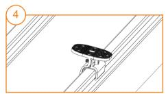
Secure the clamp by fastening the two M8\*25 inner hex bolts.
