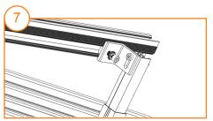
Loosely install a M8\*25 bolt and a rail nut to the leg connector and tilt the nut into rail groove.
