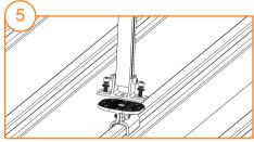
Put the leg base onto clamp, and connect them by two M8\*25 bolts.
