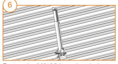
Fasten the M8\*25 inner hex bolts to secure the rear leg.
