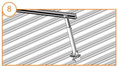
Fasten the M8\*25 inner hex bolt to connect the rail and rear leg.
