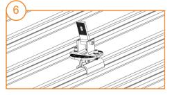
Fasten the M8\*25 inner hex bolts to secure the front leg.
