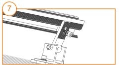
Loosely install a M8\*25 bolt and a rail nut to the leg and tilt the nut into rail groove.
