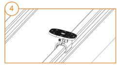
Fasten the clamp by the two M8\*25 inner hex bolts. M8: tighten torque is 15N.m; safe torque is 20N.m;
