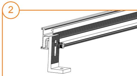
2 Install a M8\*25 inner hex bolt and a rail nut loosely onto the L foot, then tilt the nut into the rail groove. Fasten the bolt to secure the rail.
