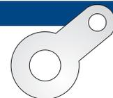
The wire is preferably soldered onto the tag part of the solder lug before assembly to minimise time to heat up the components and reduce risk of damage to the assembly.
